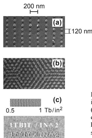
Fig. 2. Series of 40-nm data bits formed in a uniform array with (a) 120-nm and (b) variable pitch, resulting in bit areal densities of up to 400 Gb/in.<sup>2</sup>. (c) Ultra-high-density bit writing with areal densities approaching 1 Tb/in.<sup>2</sup>. From [7].
