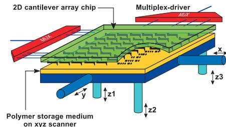
Fig. 1. Illustration of the Millipede concept. From [9].
