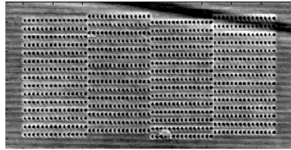
Fig. 3. A, B, C, D servo bursts. Track pitch and bit pitch set to 84 nm.
