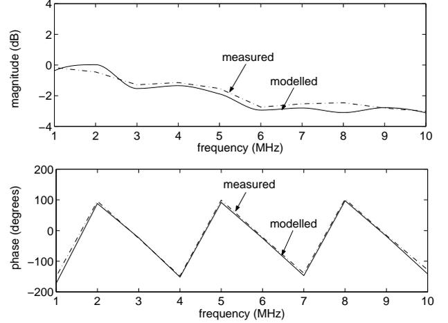
Figure 5: Measured and modelled response of a 53.3m cable line.
