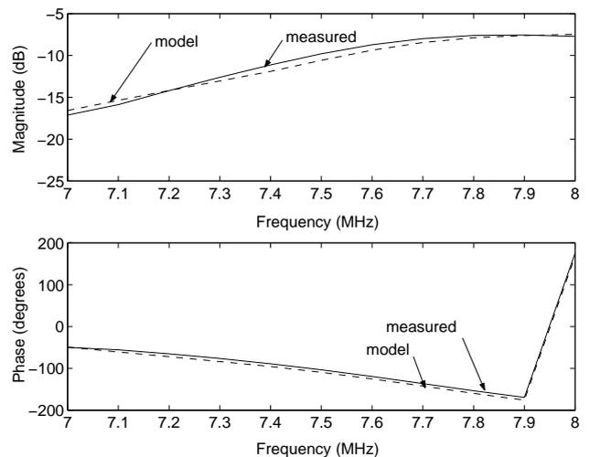
Figure 8: Measured and modelled response of the experimental network (7-8 MHz).
