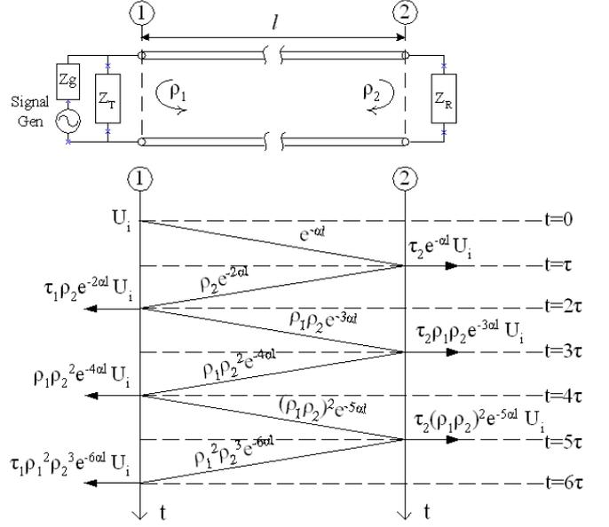
Figure 1: Timing diagram of signal propagation on a cable line.
