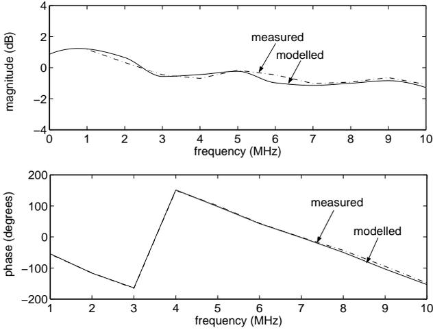
Figure 4: Measured and modelled response of a 22.3m cable line.
