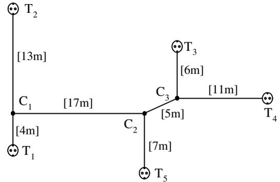
Figure 6: Experimental power line topology.
