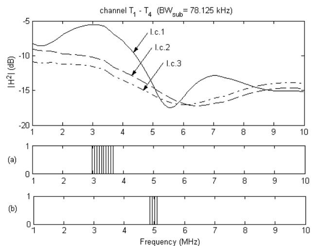
Figure 4: Unsuitable subchannels on the  $T_1 - T_4$  link.
