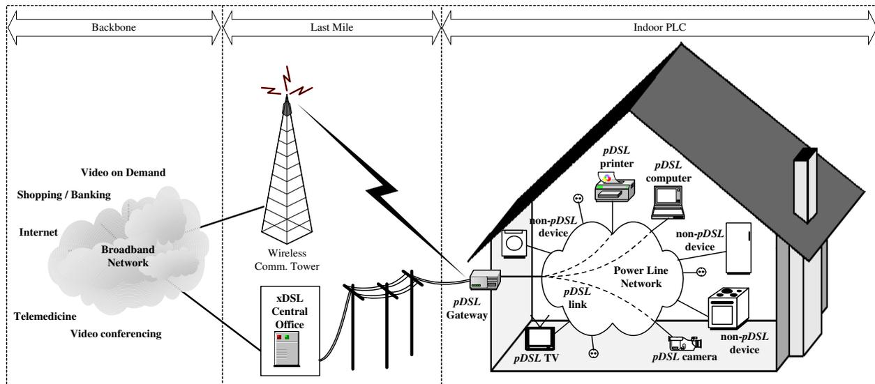
Figure 1: *pDSL* Service Structure.
