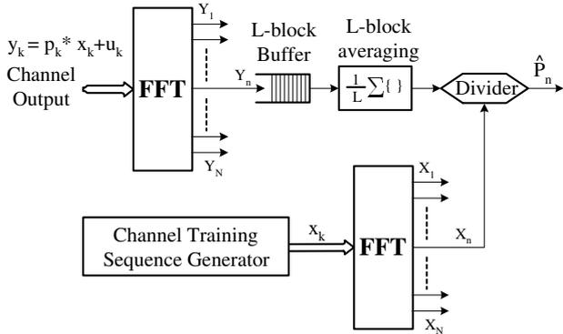
Figure 2: Functional diagram of the channel estimation process.
