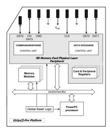
Figure 1. SD Interface Prototype Platform Architecture.
