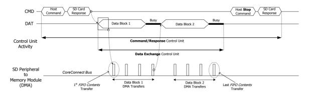
Figure 3. An example of the 'Write Multiple Block' Command in the SD Memory Card Prototype.
