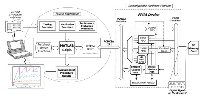
Figure 4. SD Card Interface Testing Environment.
