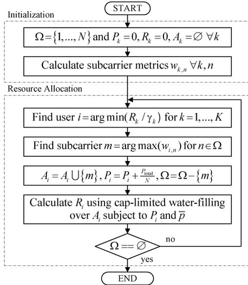
Fig. 1. Multiuser resource allocation algorithm.
