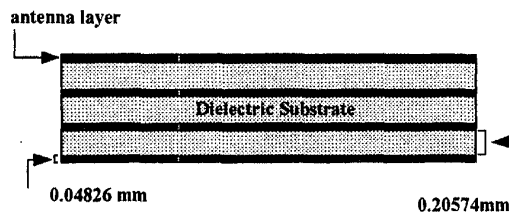
Figure 1b. A cross section of the geometry of the IFA/PCMCIA card system.
