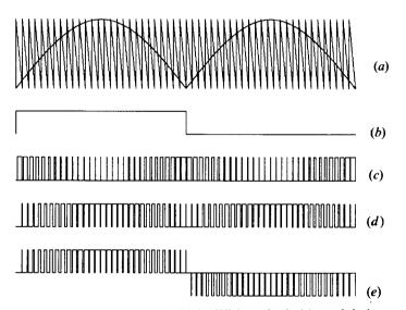
Figure 1. High switching frequency sinusoidal PWM method: (a) modulating and carrier signals; (b) polarity discriminator signal; (c) complementary PWM pulse train; (d) PWM pulse train; (e) equivalent 3-level PWM wave form.
