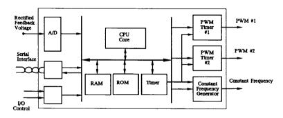
Figure 4. Block diagram of controller.
