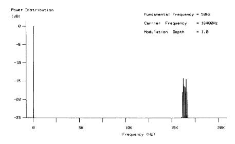
Figure 10. Harmonic analysis of HSFS-PWM method.
