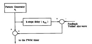
Figure 5. Internal processing operation.
