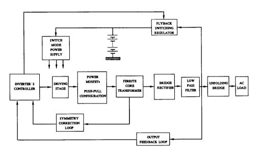
Figure 3. DC/AC power inverter block diagram.
