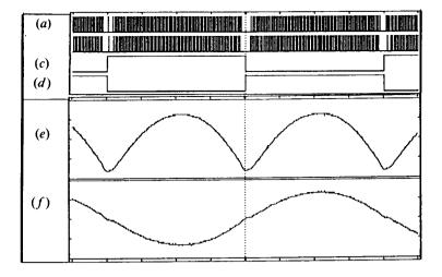
Figure 6. Sine wave generation process: (a) output of the PWM no. 1 timer; (b) output of the PWM no. 2 timer; (c) polarity discriminator signal; (d) complementary polarity discriminator signal; (e) 'folded' sine wave; (f) output sine wave (voltage: 220 V R.M.S.).
