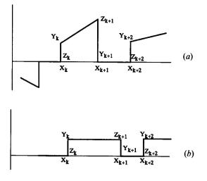
Figure 9. Piecewise linear waveform presentation and its application to a PWM pulse train (Tzou and Wu 1988).
