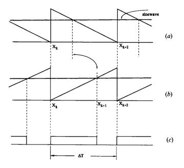
Figure 2. Details of the HSFS-PWM Method: (a) modulating and carrier signals; (b) 'intersection-position determined' method; (c) generated PWM pulse.
