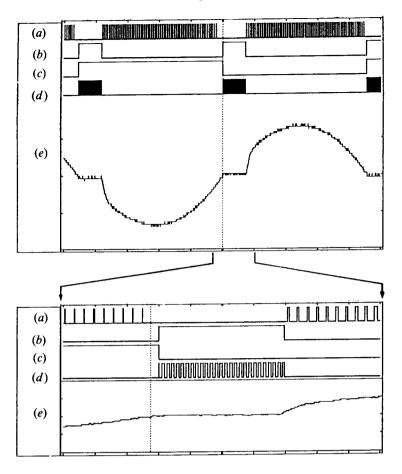
Figure 8. Inverter regeneration process: (a) PWM signal; (b) constant frequency signal; (c) polarity discriminator signal; (d) regeneration phase indicator; (e) output sine wave (voltage: 220 V R.M.S.).
