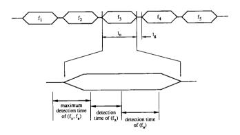
Figure 6. The '5-tone' selective signalling system.
