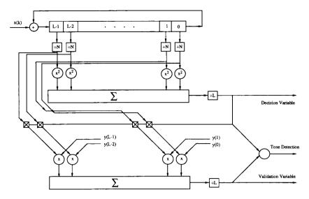
Figure 8. Block diagram of the algorithm implementation.
