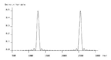
Figure 3. Decision variable versus frequency (expected frequency: 1275 Hz).
