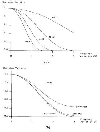
Figure 4. The value of the decision variable versus the frequency variation: (a) for various values of N; (b) for various SNR values.
