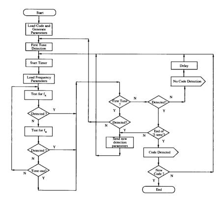
Figure 7. Flowchart of the '5-tone' selective signalling system algorithm.
