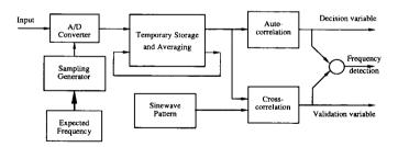
Figure 1. Block diagram of the tone detection procedure.
