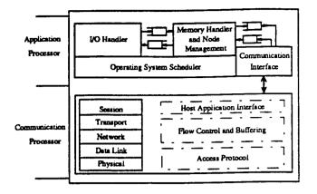
Fig. 5. The PLNode Software/Protocol Architecture
