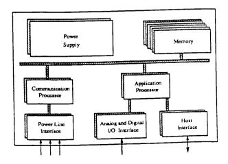
Fig. 4. The PLNode Hardware Architecture
