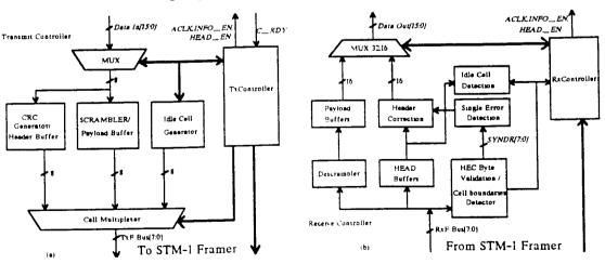
Fig. 6. The TC Sublayer components block diagram: (a) the transmitter, (b) the receiver.
