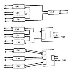
Fig. 1. CPN and LAN Configurations.
