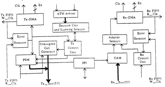
Fig. 5. The ATM Controller block diagram.
