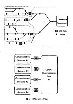
Fig. 2. The power grid structure using EMI filters and the respective communication areas.
