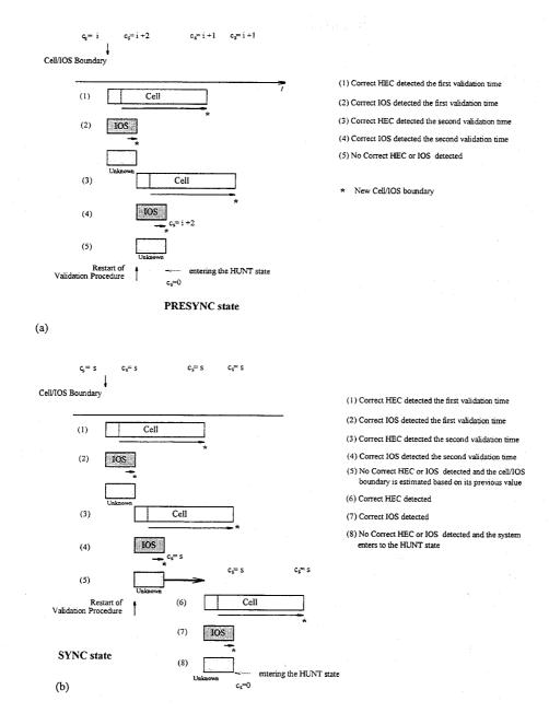
Fig. 4 Cell/IOS boundary validation procedure
