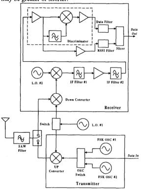
Fig. 2. The RF module block diagram
