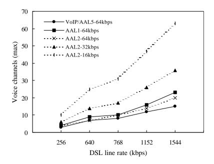
Figure 5. Number of voice channels for different DSL line rates
