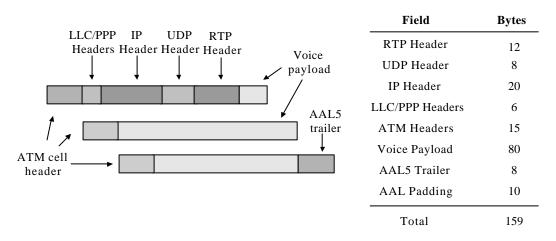
Figure 2. Packet format for VoIP/AAL5 connection with 80-byte voice payload
