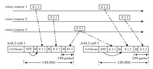
Figure 3: AAL2 cell packing
