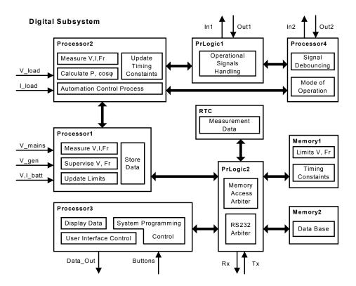
Figure 3. GCS system-level design.
