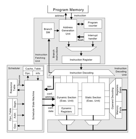
Fig. 2: The Dynamically Reconfigurable Processor Architecture
