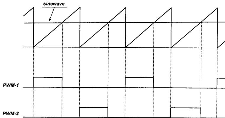
Figure 2. The PWM pulses generation process.
