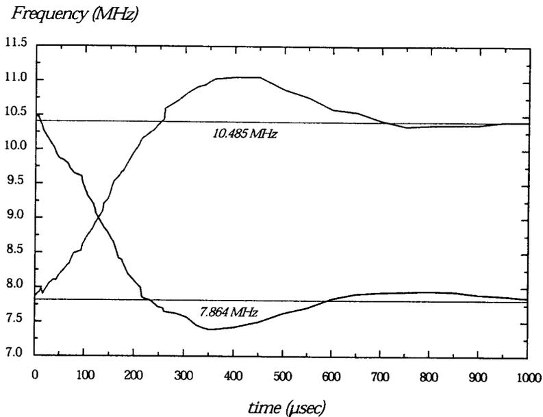
Figure 4. Clock synchronization time from 10.485 MHz to 7.864 MHz.
