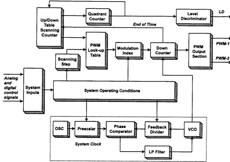
Figure 1. Modulator architecture using the internal PLL-based system clock.
