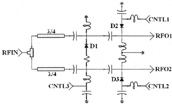
Fig. 2: The feeding network circuit.
