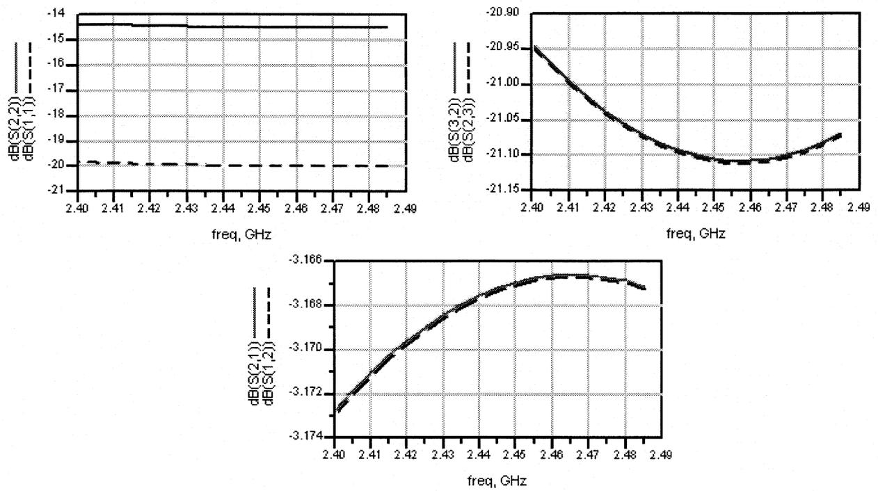
Fig. 4 S-parameters of the two-output case.
