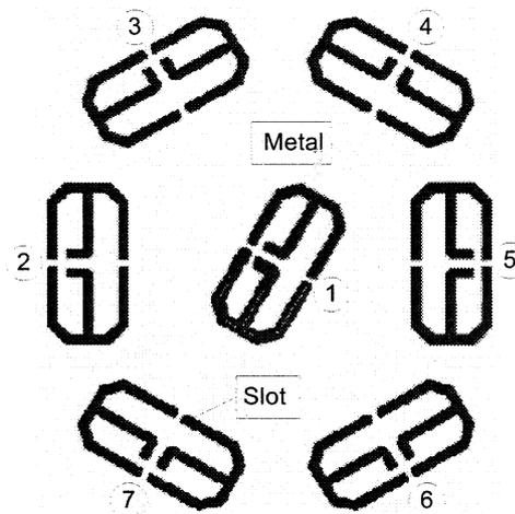
Fig. 1: The seven-elements antenna array.
