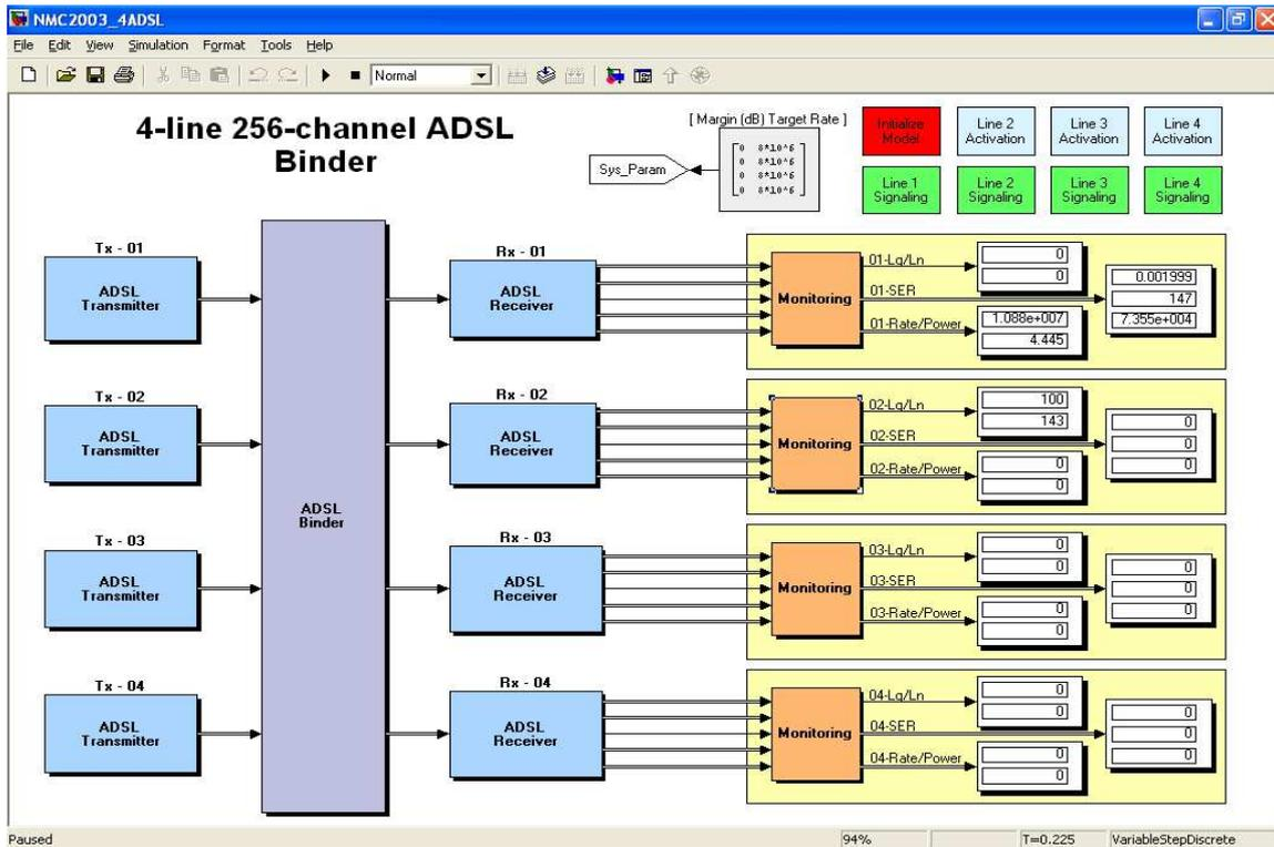
Figure 2. The 4-lines ADSL binder model in Simulink.
