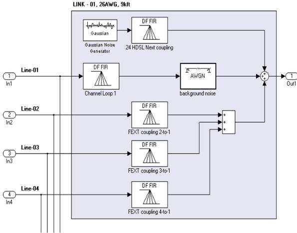
Figure 4. Part of the binder subsystem.
