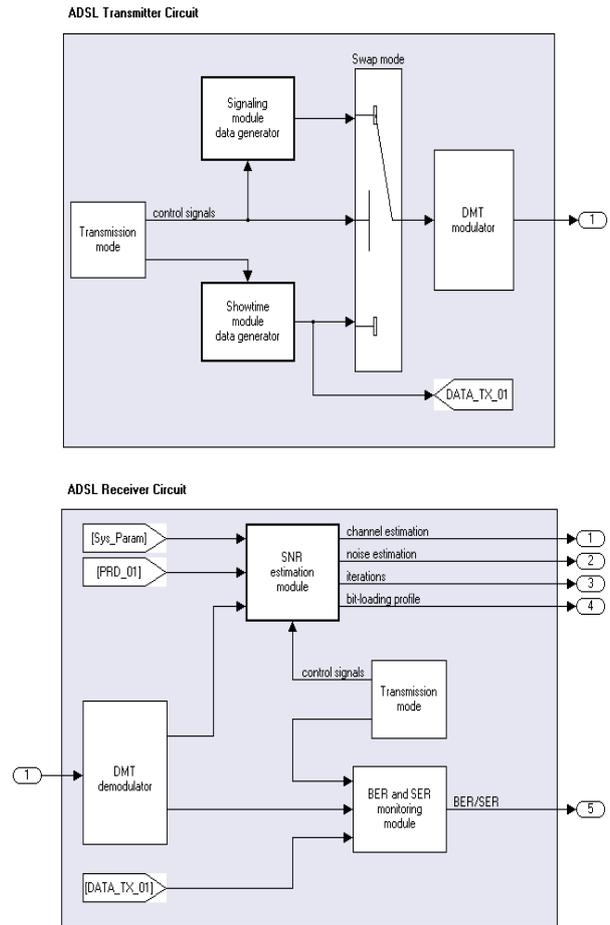
Figure 3. ADSL Tx and Rx subsystems.
