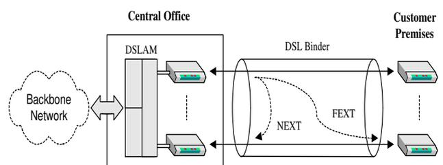
Figure 1. The DSL system architecture.
