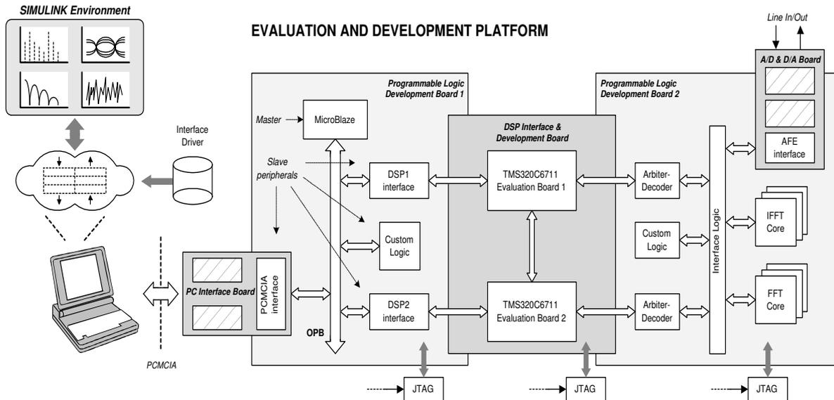
Figure 6. The mixed-level simulation and hardware development setup.
